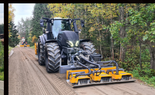
MPC-375 Gravel road compacting
