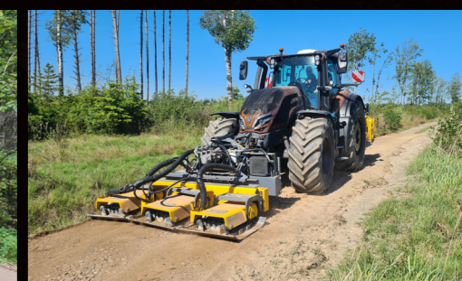
MPC-375 Forest road compacting
