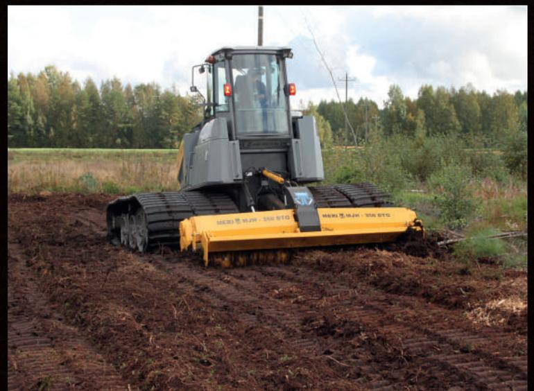
**MT-700** with steel tracks and MJH-2.4 meter crusher clearing dense vegetation. Crusher is equipped with heavy duty push bar and sizing screen.
