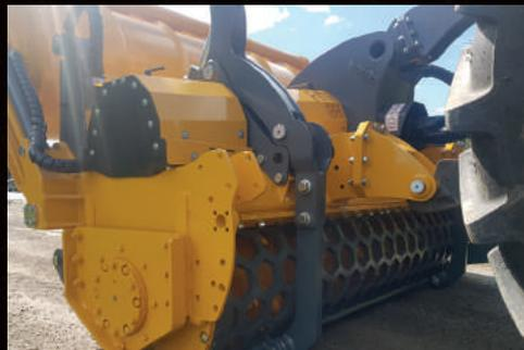
**MeriCrushers MJH and MJF** models can be equipped with patented sizing screen
