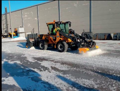
**MC4-Hydraulic** crushing of ice from parking area
